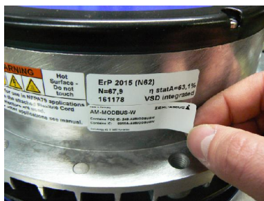
Sticking the AM-MODBUS-W inside label on the ECblue housing.
