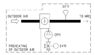
Temperature is controlled to a separate setpoint via temperature sensor after preheater (GT11).
