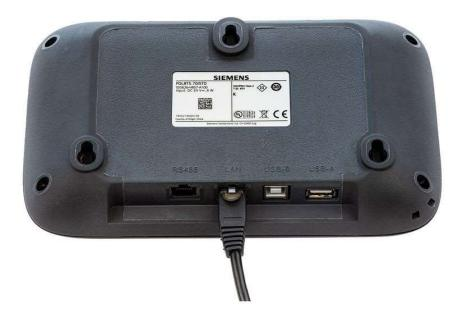
Now connect the cable from the hand-held terminal to the Climatix Ethernet TCP/IP port as shown below.
