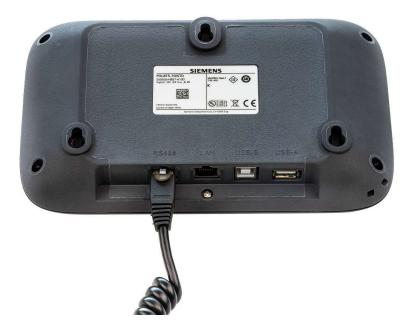
Now connect the cable from the hand-held terminal to the Climatix hand-held terminal port as shown below.
