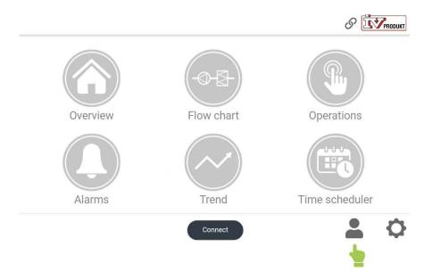
Enter the Climatix PIN (the same PIN as when logging in on hand-held terminal POL 895.50/STD) to sign in with the required authorisation level.
