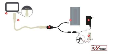
If one or more control units are connected with a network cable to the local area network in the property, one or more touch screens can be connected in a completely different part of the property via the local area network according to example 2.
